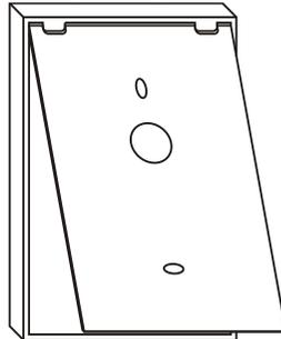
3. Attach the backplate to the wall using screws in the two oval mounting holes and drill out a hole for the cable.
